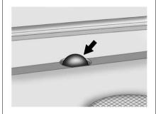
The solar sensor located on the instrument panel, near the windshield, monitors the solar heat.
